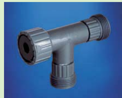
TKA Distribution manifold Made of plastic. 1 inlet, 2 outlets to which shutoff and distributing taps can be connected. R 3/4" connectors. No. 03.1420
