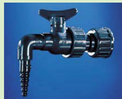
TKA Purified water outlet tap Made of plastic, angled. Connector R 3/4", coupling nut. Dimensions: 50 x 90 x 140 mm. No. 03.1401
