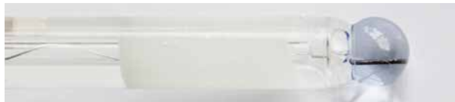
③ Blue pH glass bulb of a pH electrode
