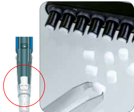
Pipette contamination in pipette barrel when pipetting liquid culture of bacteria Micrococcus Luteus .
