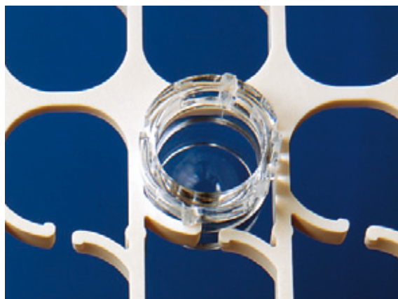
The LockWell™ frame has a unique spring lock. It locks each individual well in the frame through an undercut in the well. The spring lock does not touch the strip or well when inserted in the frame
