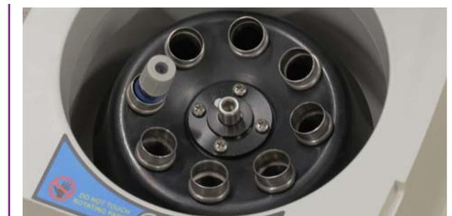
4 | Metal angle rotor (autoclavable) and plastic tube holders.
