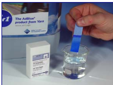
Remove the test paper. A dark coloration indicates the presence of fuel.
