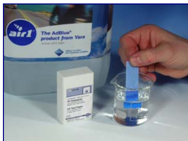
Move test paper back and forth 3-5 times.
