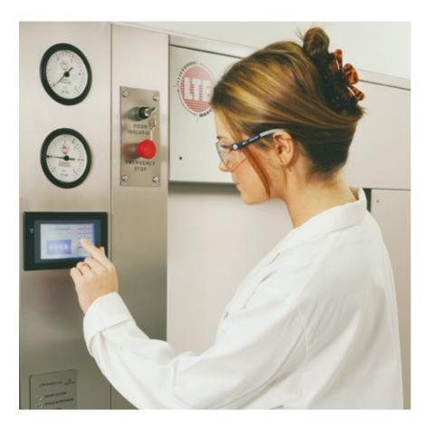
Labclave 23 is LTE Scientific's low-cost 23-litre laboratory autoclave. Designed to offer effective and fast sterilization of many laboratory load types and taking up a floor area of just 460mm x 395mm, Labclave 23 has to be one of the most compact units available.
