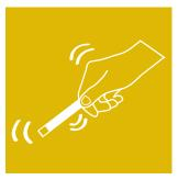
2. Shake the strip to remove any excess solution. In some tests this step may not be necessary.
