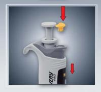
Remove the calibration key and set the calibration switch in its lower position. Place the cap on the ejector button.
