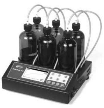
Use the Hach BODTrak II Apparatus for unattended, fast BOD (Biochemical Oxygen Demand) analysis. Features include delayed start for temperature stabilization, continuous data readout, and automatic shut-off.
