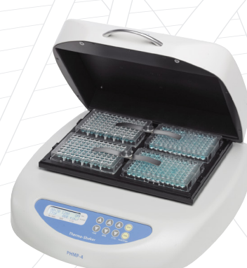
PHMP-4 thermoshaker for four microplates
