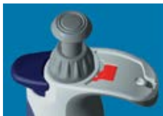
Red recalibration flag indicates adjustment from factory specifications.
