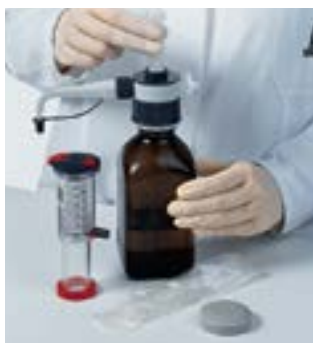
Sterile dispensing cartridge installation
