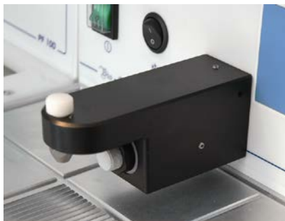
Dispensing nozzle controlled by proximity sensor.
