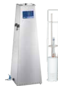
SONOREX PR 140 DH - Ultrasonic bath for cleaning volumetric glassware
