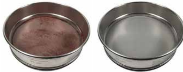
Test sieve before and after cleaning
