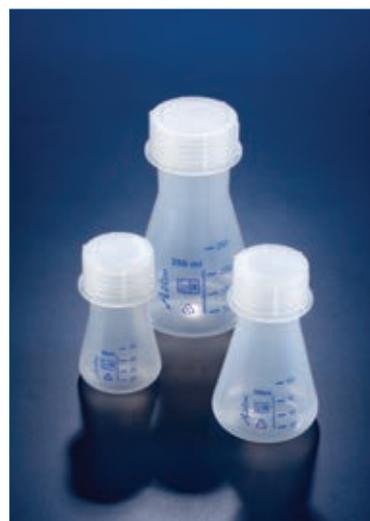
**i** When autoclaving flasks always ensure the caps are completely loosened to prevent accidental implosion.
