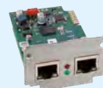
LRZ 923 EtherCAT module with RJ45 connection
