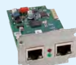
LRZ 923 EtherCAT module with RJ45 connection
